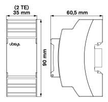
Figure 3. H10-XP Circulation Pump Control, H10-XS Heating/Cooling Demand, H10-XW 1-Wire® Bridge Extension Modules - Dimensions
