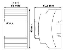
Figure 2. H10/230-XI Wired 230V~/50Hz, H10/24-XI Wired 24V Thermostat Interface Extension Modules – Dimensions
