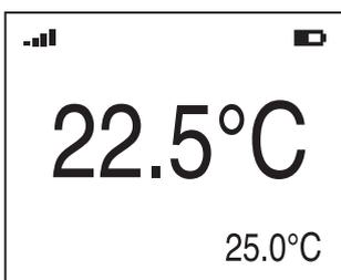
10. After joining a network successfully, the display will show the current target room temperature (center) and the actual room temperature (bottom right).
